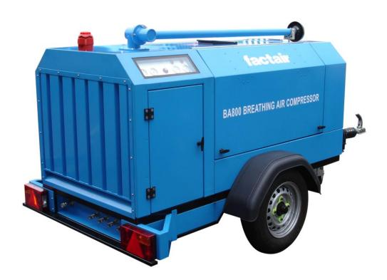
range of demanding environments with a sand trap louvre ventilation and a specially uprated cooling system allowing the units to operate in both hot and dusty conditions. In addition, as standard, the units are fitted with Chalwyn valve, spark arrestor and a high-level air intake to ensure that air is drawn in from an area clear of exhaust gases.
