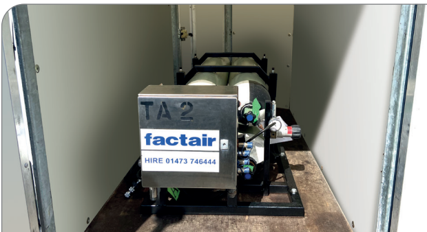
4 CYLINDER – LONG DURATION BREATHING-AIR UNIT
