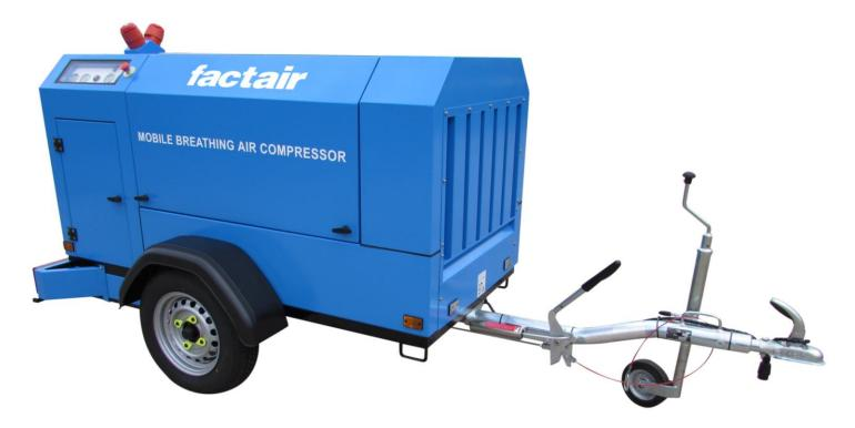
The BA800E will produce up to 800 I/min at 8 bar and incorporates breathing-air filtration with a pressure swing dryer CO and CO<sub>2</sub> suppression system. The unit incorporates FACTAIR's 'fail-safe' system providing automatic back up from high-pressure cylinders, ensuring a safe exit from the workplace in the event of failure of the primary supply.
