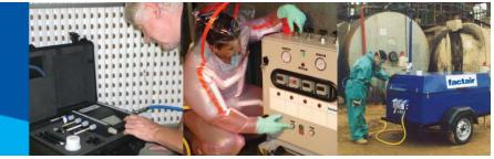
Factair's trailer mounted breathing-air centres are specially designed to provide safe breathing-air for operatives working in hazardous environments.
