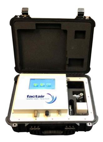
Test results are saved in the instrument's memory and can then be downloaded, to PC software provided with the instrument.
