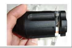
3. Place your used detector tubes in the F2154 Travel Container, until they can be disposed of properly as "sharps" or glass.
