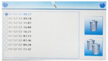
The F6001 can store up to 20 test results and each individual test is titled by the date and time when the test was completed.
