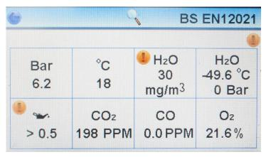
If the test was a fail an orange exclamation mark would be indicating those criteria which did not meet the standard. The photograph opposite is an example of a failed test where the F6001 was testing a high pressure charging compressor and the air quality for water and oil did not meet the requirements of breathing-air standard BS EN 12021.
