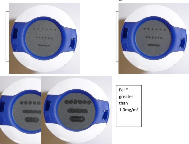
\* – The above pass and fail criteria is based on breathing-air standard EN12021 Using the Draeger tube tip cutter
