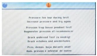
This error message will be displayed when the air inlet pressure has fallen below the minimum 2 bar required for the instrument to successfully complete the test. The test will need to be restarted with a pressure greater than 2 bar.
