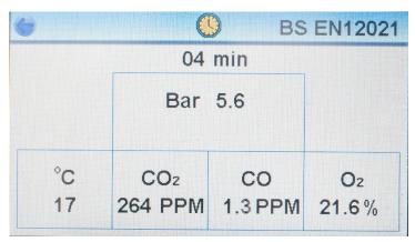
The test will now commence and the duration will be displayed as a countdown, together with pressure, ambient temperature, carbon dioxide, carbon monoxide and oxygen content.
