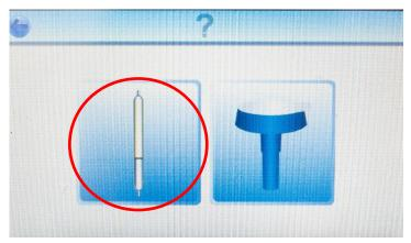
To complete a tube test commence a new test and after the unit had calibrated the oxygen cell and you have input the test location details you will have the option to select a tube test as shown, press the button to proceed.
