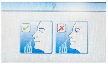
Carry out the odour test by depressing the odour test button and smelling the air exhausted from the sintered outlet, then release the button. If there is a serious odour problem, fail the sample at this point of the test. Initiating flows of seriously contaminated air through the tube ports could result in damage to the unit. If the odour test is satisfactory, press the 'pass' icon.
