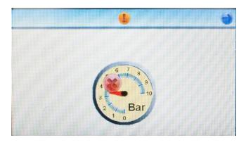
This message will be displayed prior to the test when the instrument is unable to calibrate the oxygen cell because there is an air supply connected to the instrument. Disconnect the air supply then press the arrow button in the top right hand corner to continue.
