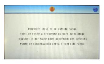
This reading will be displayed during the test if the moisture reading falls outside the range of the sensor (-70 to 0°C atmospheric dewpoint). The final test result for moisture will therefore display the limit for the sensor.
