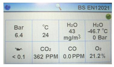
The "test complete" screen displays all the measurements recorded during the test. And automatically determines whether the test was a pass or fail against the standard displayed in the top right corner of the screen. For water content on high pressure tests both the measured value in mg/m³ and the atmospheric dewpoint are provided.
