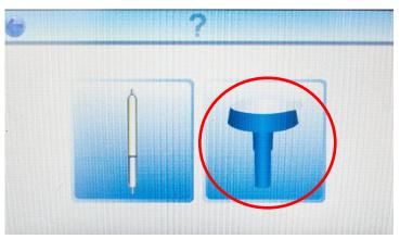
Choose between using a Draeger chemical reagent tube or Draeger oil Impactor in the test port.
