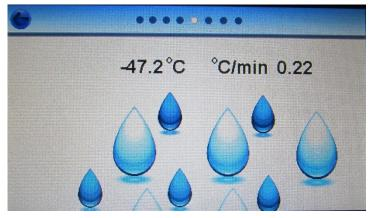
If the instrument detects that the dewpoint meter's rate of change is still too high (>0.2 dec C per minute) it will automatically continue the test until this stabilises (maximum test time 15 minutes).
