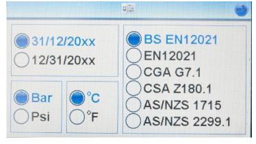
In this menu you can then choose date format; pressure and temperature units of measure and the breathing-air test standard.
