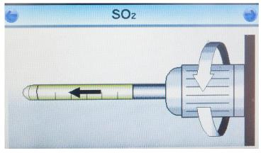
Once you have selected which tube you wish to test the instrument will complete its purge sequence after which you will be prompted to insert the appropriate tube into the test port and tighten firmly.
