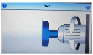
Once the purge has finished, the Draeger Impactor should be inserted into the test port and tightened firmly; ensure the Impactor has an intact protective seal. This seal must remain in place for the duration of the test. Press the button in top right hand corner to start the test.
