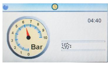
The instrument will now commence a 7-minute purge sequence, during which time an airflow will be passed through the test port and across the electronic cells. This clears contaminants from previous tests and ensures that a representative sample is being tested.
