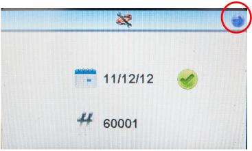
A Stylus pen is provided for use with the touch screen. The display will show the, date last calibrated, serial number and a tick or cross symbol will indicate whether it is within the recommended calibration period.
