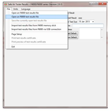
Individual test records can be opened from the file drop down menu by selecting "Open an F6000 test results file".
