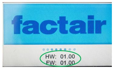
A splash screen will be displayed which shows the instruments hardware and firmware versions. Periodically the firmware is upgraded as part of the recalibration process as improvements are identified.
