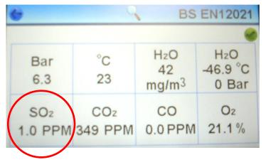
The result will then be displayed on the final test result screen and stored in the instrument's memory. In the example opposite a sulphur dioxide tube has been used.
