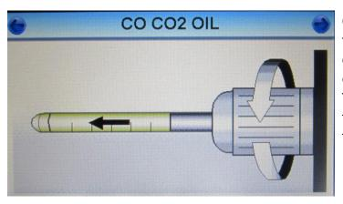
Once the purge has finished, the Draeger tube/Impactor should be inserted into the corresponding test port and tightened firmly; ensure the Impactor has an intact protective seal. This seal must remain in place for the duration of the test. Press the button in top right hand corner to start the test.
