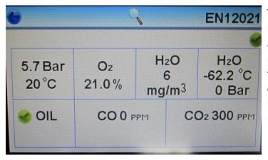
The "test complete" screen displays all the measurements recorded during the test. And automatically determines whether the test was a pass or fail against the standard displayed in the top right corner of the screen. For water content on high pressure tests both the measured value in mg/m³ and the atmospheric dewpoint are provided.
