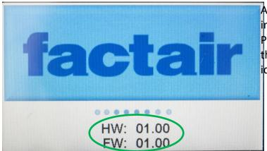
A splash screen will be displayed which shows the instruments hardware and firmware versions. Periodically the firmware is upgraded as part of the recalibration process as improvements are identified.
