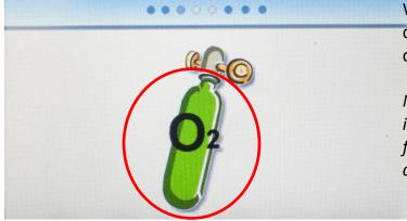
When you start a test press and hold the O2 cylinder for a few seconds which it is in its self calibration mode.
