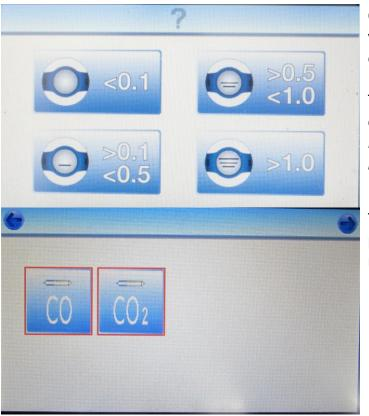
Once the test is complete close the flow control valve, the readings from the Impactor can now be entered.
