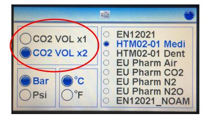
When entering the test results into the tester, the tube reading shall automatically be divided by two, to reflect the actual rending as shown below.
