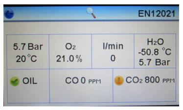
If the test was a fail an orange exclamation mark would be indicating those criteria which did not meet the standard. The photograph opposite is an example of a failed test where carbon dioxide failed to meet the requirements of the selected standard.
