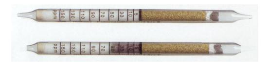
The standard CO tube (67 28511) has a range of 0 to 150 PPM, and the maximum limit for medical air in Pharmacopeia is 5 PPM.
