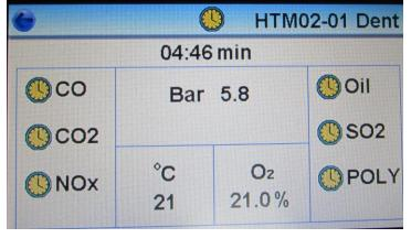
The test will now commence and the duration will be displayed as a countdown, together with test standard. The pressure, ambient temperature, and oxygen content will also be displayed.
