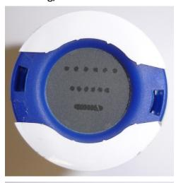
Fail / (Pass for EN12021 breathing-air only) - greater than 0.1mg/m³ but less than 0.5mg/m³
