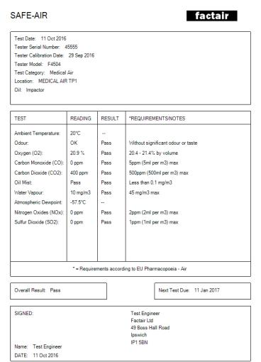
In the UK, for breathing-air tests the Health and Safety Executive guideline HSG53 recommends test results should be retained for a minimum of 5 years.
