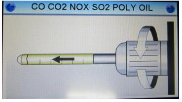
Once the purge has completed the chemical reagent tubes / Impactor should be inserted into the corresponding test port and tightened firmly. The tubes/Impactors to be used are shown at the top of the screen and will be dependent on the test standard selected earlier.
