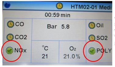
Depending on the standard and therefore the chemical reagent tubes / Impactor being used some will complete at different test times and the instrument will automatically stop the flow to these tubes. Each complete test port will be shown with a green tick.
