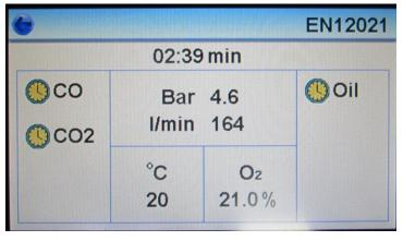
The test will now commence and the duration will be displayed as a countdown, together with pressure, flowrate, ambient temperature, carbon dioxide, carbon monoxide and oxygen content.
