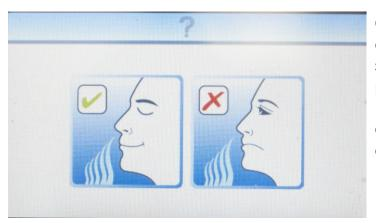
Carry out the odour test and smell the air exhausted from the sintered outlet. If there is a serious odour problem, fail the sample at this point of the test by pressing the 'fail' button. Initiating flows of seriously contaminated air could result in damage to the instrument. If the odour test is satisfactory, press the 'pass' button.
