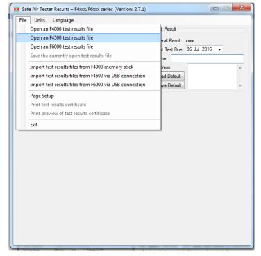
Individual test records can be opened from the file drop down menu by selecting "Open an F4500 test results file".
