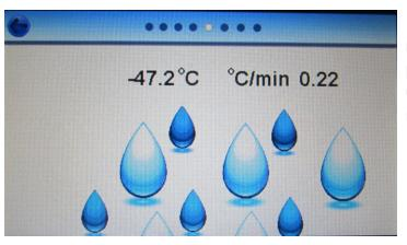
If the instrument detects that the dewpoint meter's rate of change is still too high (>0.2 dec C per minute) it will automatically continue the test until this stabilises (maximum test time 15 minutes).
