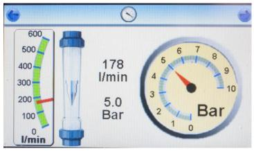
We can now confirm the flow and pressure is adequate for your respiratory protective device. Adjust the system's flow control valve so that the flow meter registers the required level\*, check the pressure is sufficient for the breathing-air equipment being used. It is recommended that this flow is left running for the duration of the test to simulate the conditions of use. Press the arrow key to proceed if the flow and pressure meet the minimum requirements for your RPD.
