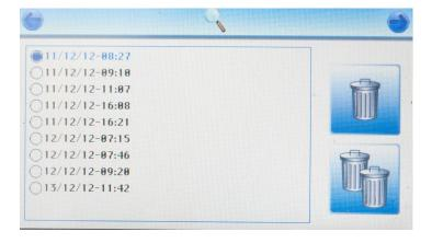
The F4504 can store up to 20 test results and each individual test is titled by the date and time when the test was completed.
