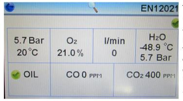
The "test complete" screen displays all the measurements recorded during the test. And automatically determines whether the test was a pass or fail against the standard displayed in the top right corner of the screen. The water content on low pressure tests is displayed as a pressure dewpoint. The test result is recorded in the instrument's memory, which can store up to 20 previous tests.
