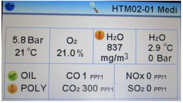
The "test complete" screen displays all the measurements recorded during the test. And automatically determines whether the test was a pass or fail against the standard displayed in the top right corner of the screen. The water content is automatically also displayed, together with oxygen content, ambient temperature and test pressure. The test result is recorded in the instrument's memory, which can store up to 20 previous tests.
