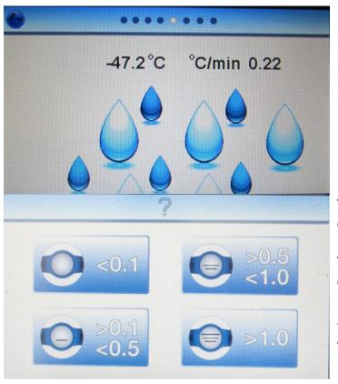
If the instrument detects that the dewpoint meter's rate of change is still too high (>0.2 dec C per minute) it will automatically continue the test until this stabilises (maximum test time 15 minutes).
