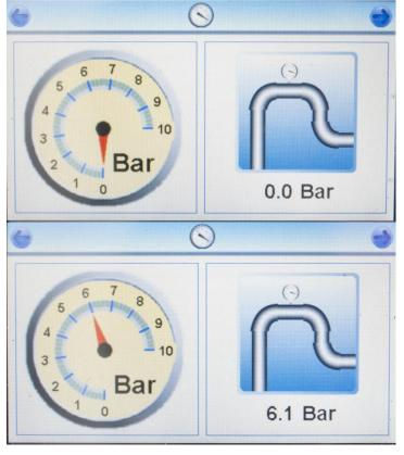
With the flow control valve in the closed position connect to the air supply to be tested. Ideally this should be done by using the hose which normally supplies the breathing apparatus. Fit the appropriate adaptor to the Tester first and then connect the supply hose to the adaptor.
