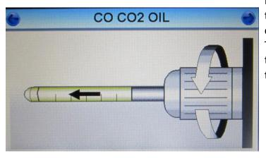
Once the purge has finished, the CO, CO<sub>2</sub> and Draeger Impactor/oil tube should be inserted into the corresponding test port and tightened firmly; ensure the Impactor has an intact protective seal. This seal must remain in place for the duration of the test. Press the button in top right hand corner to start the test.
