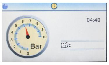
The instrument will now commence a 5-minute purge sequence, during which time an airflow will be passed through the test port and across the electronic cells. This clears contaminants from previous tests and ensures that a representative sample is being tested.
