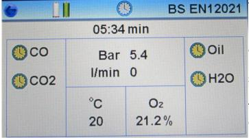
The test will now commence and the duration will be displayed as a countdown, together with pressure, flowrate, ambient temperature and oxygen content.
