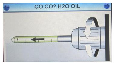
Once the purge has finished, the Water (F4500 only), CO,  $CO_2$  and Draeger Impactor/oil tube should be inserted into the test port and tightened firmly; ensure the Impactor has an intact protective seal.
