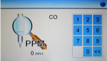
Input the reading from the tube and press the arrow icon in the top right hand corner of the screen.
