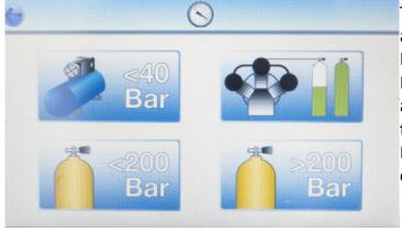
The unit has 4 breathing-air test programmes available: Airline Systems up to 40 bar (top left); High Pressure Charging Compressors (top right) High Pressure Systems up to and including 200bar and High Pressure Cylinders above 200bar. All of the high-pressure tests require the use of the F3002 regulator which has a DIN connector that can accept input pressures up to 300bar.
