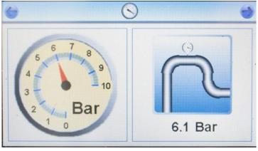
Note:- If the unit is over-pressurised it will automatically shut down and display an overpressure warning; it will then need to be returned to the manufacturer for checking and resetting.
