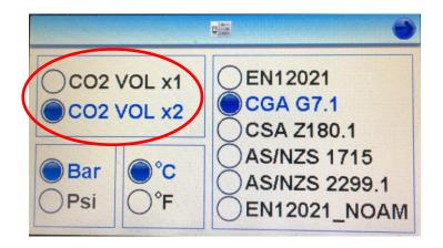
For the CO<sub>2</sub> tube (67 28521), there is an option to adjust the test volume up by a factor of two to increase the number of scale points. This option can be set within the setup menu as shown here.
