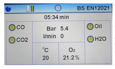
The test will now commence and the duration will be displayed as a countdown, together with pressure, flowrate, ambient temperature and oxygen content.
