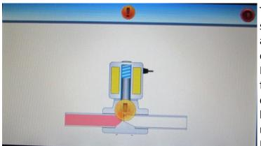
The F4500 incorporates a unique flow checking system to ensure that the air is passing through all 4 outlet ports, thus eliminating the possibility of a false positive result.
