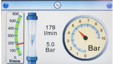
We can now confirm the flow and pressure is adequate for your respiratory protective device. Adjust the system's flow control valve so that the flow meter registers the required level\*, check the pressure is sufficient for the breathing-air equipment being used. It is recommended that this flow is left running for the duration of the test to simulate the conditions of use. Press the arrow key to proceed if the flow and pressure meet the minimum requirements for your RPD.
