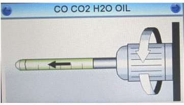
Once the purge has finished, the Water (F4500 only), CO,  $CO_2$  and Draeger Impactor/oil tubes should be inserted into the test ports and tightened firmly; ensure the Impactor has an intact protective seal.
