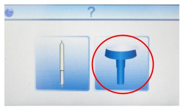
Choose between using a Draeger chemical reagent tube or Draeger Oil Impactor in the test port.
