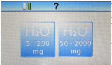
The F4500 can be configured with the Draeger 6728531 water tube for 2 different scales. Select the appropriate water range: 50 to 2000 mg/m³ is for standard airline systems with a fridge dryer or no dryer and 5 to 200 mg/m³ is for systems incorporating desiccant dryers. Having selected the appropriate range press the arrow key.
