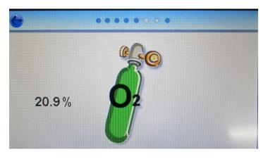
The instrument will then change operating modes to continuously display the oxygen reading, connect your air source and the instrument will continue to provide a reading until you press the arrow key in the top corner.
