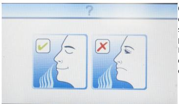
Carry out the odour test and smell the air exhausted from the sintered outlet. If there is a serious odour problem, fail the sample at this point of the test by pressing the 'fail' button. Initiating flows of seriously contaminated air could result in damage to the instrument. If the odour test is satisfactory, press the 'pass' button.
