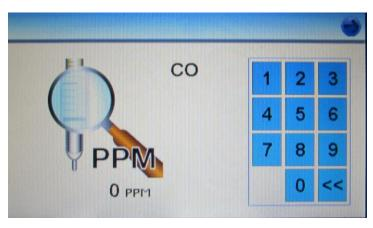
Input the reading from the tube and press the arrow icon in the top right hand corner of the screen.
