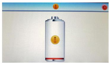
Should mains power not be connected and both battery sources low, a battery icon shall be displayed on-screen and it will not be possible to proceed with a test.
