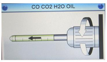
Once the purge has finished, the Water (not ED version), CO,  $CO_2$  and Draeger Impactor/oil tubes should be inserted into the appropriate test ports and tightened firmly; ensure the Impactor has an intact protective seal.
