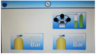
The unit has 3 breathing-air test programmes available: High Pressure Charging Compressors (top right) High Pressure Cylinders up to and including 200bar and High Pressure Cylinders above 200bar. All of the high-pressure tests require the use of the F3002 regulator which has a DIN connector that can accept input pressures up to 300bar.
