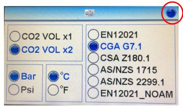
In this menu you can then choose the following; CO<sub>2</sub> sample rate, pressure and temperature units of measure and the breathing-air test standard.
