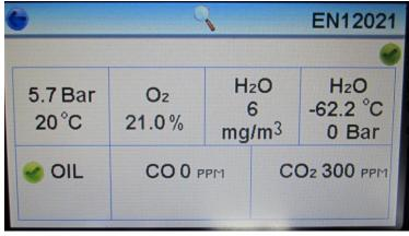
The "test complete" screen displays all the measurements recorded during the test. And automatically determines whether the test was a pass or fail against the standard displayed in the top right corner of the screen. For water content on high pressure tests both the measured value n mg/m<sup>3</sup> and the atmospheric dewpoint are provided.
