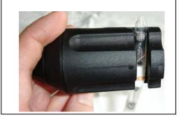
3. Place your used detector tubes in the F2154 Travel Container, until they can be disposed of properly as "sharps" or glass.
