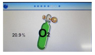
The instrument will then change operating modes to continuously display the oxygen reading, connect your air source and the instrument will continue to provide a reading until you press the back arrow key in the top corner.
