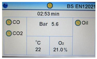
The test will now commence and the duration will be displayed as a countdown, together with regulated pressure, ambient temperature and oxygen content.
