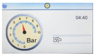
The instrument will now commence a 5-minute purge sequence, during which time an airflow will be passed through the test port and across the electronic cells. This clears contaminants from previous tests and ensures that a representative sample is being tested.
