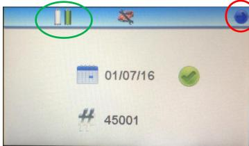
A stylus pen is provided for use with the touch screen. The display will show the, date last calibrated, serial number and a tick or cross symbol will indicate whether it is within the recommended calibration period.
