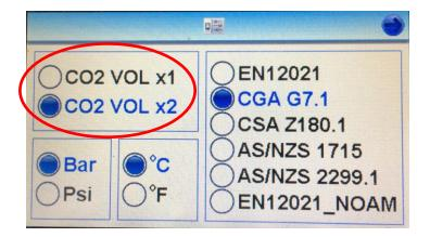
When entering the test results into the tester, the tube reading shall automatically be divided by two, to reflect the actual reading as shown below.
