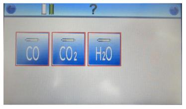
The tube readings should also then be entered, push the button corresponding to each chemical reagent tube.
