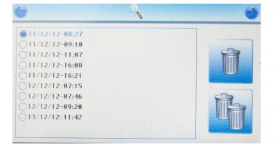
The F4501 & F4501ED can store up to 20 test results and each individual test is titled by the date and time when the test was completed.
