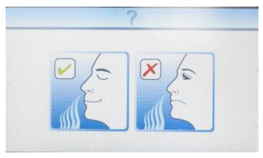
Carry out the odour test by depressing the odour test button and smelling the air exhausted from the sintered outlet. If there is a serious odour problem, fail the sample at this point of the test. Initiating flows of seriously contaminated air through the tube ports could result in damage to the unit. If the odour test is satisfactory, press the 'pass' icon.
