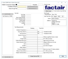
To transfer the datalog from the Safe-Air Tester to the PC software, turn on the F8104, connect the USB cable between the F8104 and your PC and open the Safe-Air Tester Results F8000 series software.
