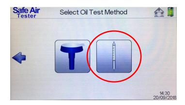
To complete a tube test, select a tube test option as shown, press the button to proceed.
