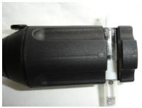
cutter, the other holding the tube and with your thumb against the base of the cutter, apply pressure to the tube, this should break the inner tube.
