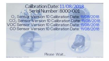
A stylus pen is provided for use with the touch screen. The display will show the calibration date, serial number and check the status of each sensor. Once each sensor status has been checked follow the touch screen prompt on screen to proceed.
