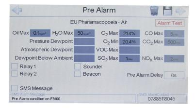
The Pre Alarm screen provides the option to set a lower alarm value which can be used to notify the user before the main alarm values are exceeded.
