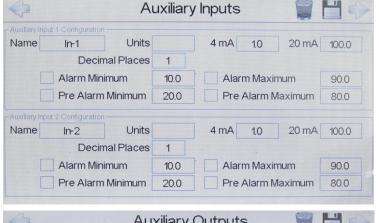
The F8104 can display readings from external sensors which have a 2 wire, 15V, 4 - 20 mA output.
