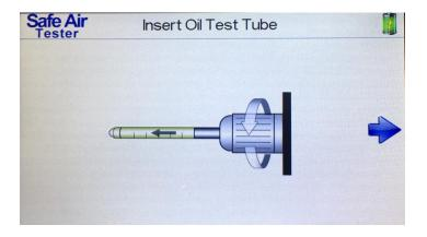
Once the instrument has completed its purge sequence you will be prompted to insert the tube into the test port and tighten firmly.
