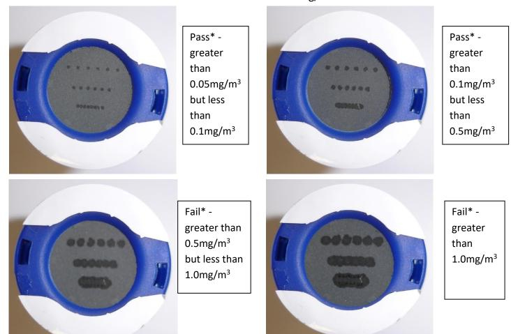
\* – The above pass and fail criteria is based on breathing-air standard EN12021
