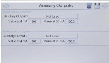
It is also possible to program 4-20mA outputs for 2 of the F8104 sensors. These can be used if you need remote indication for these sensor values.
