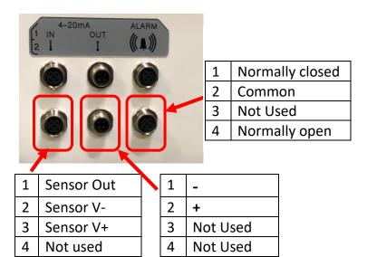
Relay 1 and 2 are used to set each alarm. These correspond with the alarm output connections located at the bottom of the instrument.
