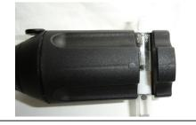
2. With one hand holding the cutter, the other holding the tube and with your thumb against the base of the cutter, apply pressure to the tube, this should break the inner tube.
