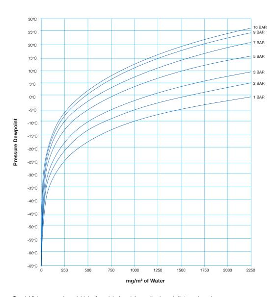
To establish pressure dewpoint take the point where tube reading in  $mg/m^3$  intersects system pressure and read off pressure dewpoint from vertical scale.
