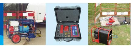
The Factair BF80E 230V single phase electric fibre blowing compressor has been specially designed to deliver clean dry air for installation of optical fibre in conjunction with either the BT 4A/4B or FIG Blowing Head Systems.
