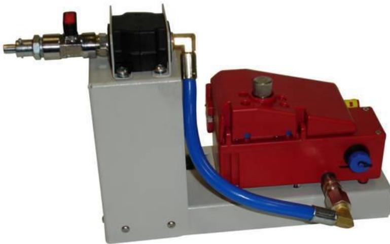
4A Blowing Head mounted on dispenser.
