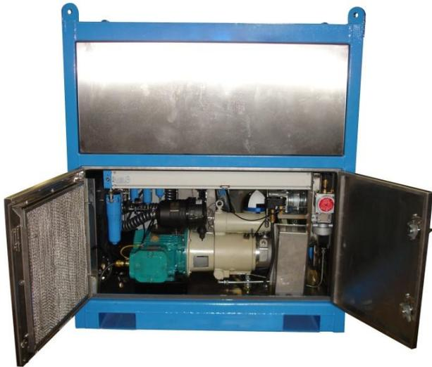
Zone 1 Breathing-Air Compressor incorporating Mattei M80E rotary vane compressor, producing 450 l/min at 7 bar from 50 Hz supply or 600 l/min at 7 bar from 60 Hz supply, dual wound motor 400V – 3ph-50Hz, 460V - 3ph-60Hz
