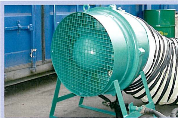
600mm Diameter Compressed-Air Powered Fan
