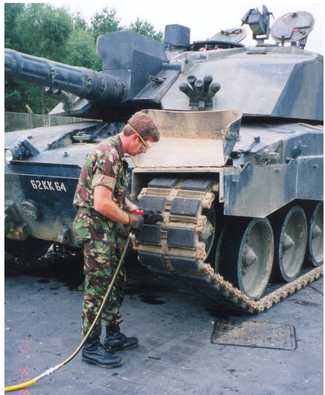
Air powered needle scaler at work on a Challenger 2 Main Battle Tank
