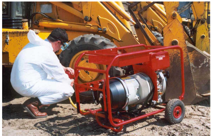
A diesel engine driven unit fitted with a pneumatic wheel kit and tool tray being used to tighten the wheel nuts of an earth mover.
