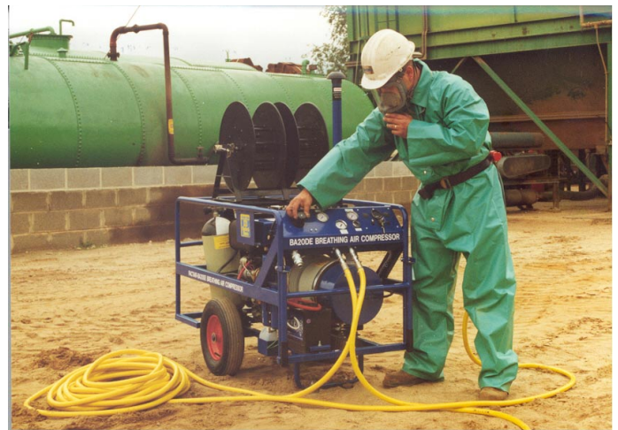
Final checks on a BA20DE mobile breathing air compressor prior to entering an oil storage tank.
