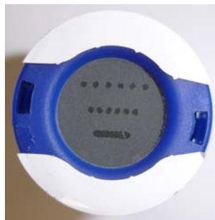
Typical Test Result – Oil present at a concentration of greater than 0.1 mg/m 3 but less than 0.5 mg/m 3
