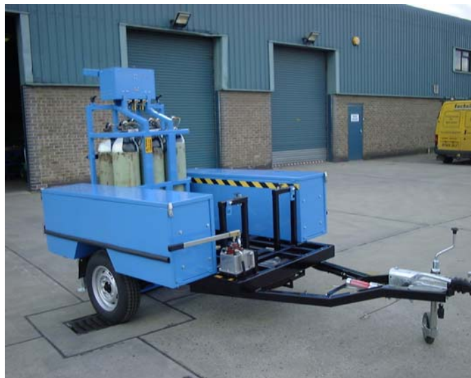
Special Trailair with hydraulic cradle rotation system and side storage pods
