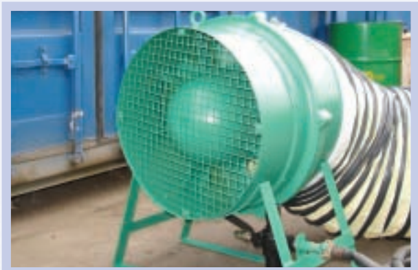
600mm Diameter Compressed-Air Powered Fan
