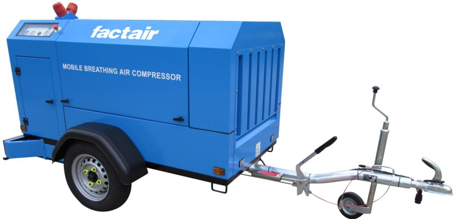
The BA800E will produce up to 800 l/min at 8 bar and incorporates breathing-air filtration with a pressure swing dryer CO and CO<sub>2</sub> suppression system. The unit incorporates FACTAIR's 'fail-safe' system providing automatic back up from high-pressure cylinders, ensuring a safe exit from the workplace in the event of failure of the primary supply.
