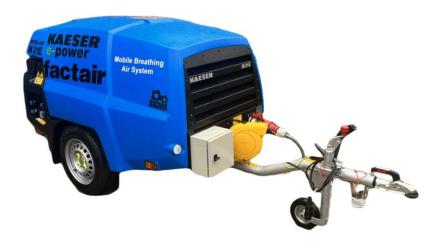
applications. The compressed air supplied is purified to breathing air standard by a 5-stage filtration and drying system that will provide breathing quality air well in excess of the criteria stated in EN: 12021: 2014, dry to a - 40°C pressure dewpoint and provide active suppression of CO and CO<sub>2</sub>.
