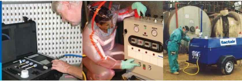
Factair pioneered air-scouring of water mains and the PS150D is the latest generation fast towing unit with all components enclosed by a weather-proof, noise attenuated enclosure.
