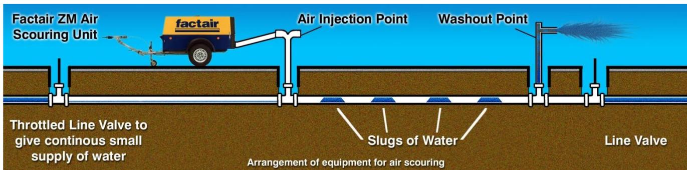
Provided with a continuous supply of compressed air and water in the right proportions, discrete slugs of water are formed in the main and are driven along at high velocity by the compressed air. It is the slug flow system that enables solids to remain suspended in the water over the long distances being cleaned.
