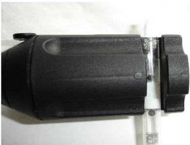
2. With one hand holding the cutter, the other holding the tube and with your thumb against the base of the cutter, apply pressure to the tube, this should break the inner tube.
