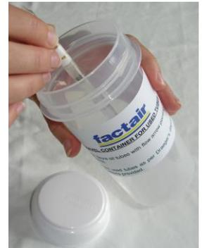
Ensure the oil tube is kept vertical throughout this process.
