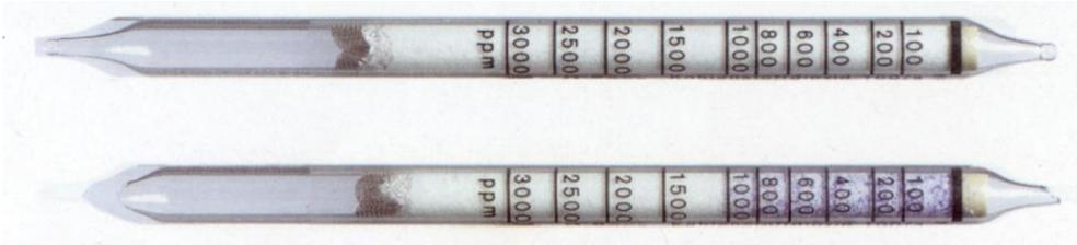
For the CO<sub>2</sub> tube (67 28521), there is an option to adjust the test volume up by a factor of two to increase the number of scale points. This option can be set within the setup menu as shown below.
