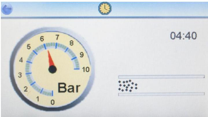
The instrument will now commence a 5-minute purge sequence, during which time an airflow will be passed through the test port and across the electronic cells. This clears contaminants from previous tests and ensures that a representative sample is being tested.
