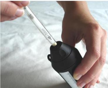
2. Push the tube at an angle to break the tip.
