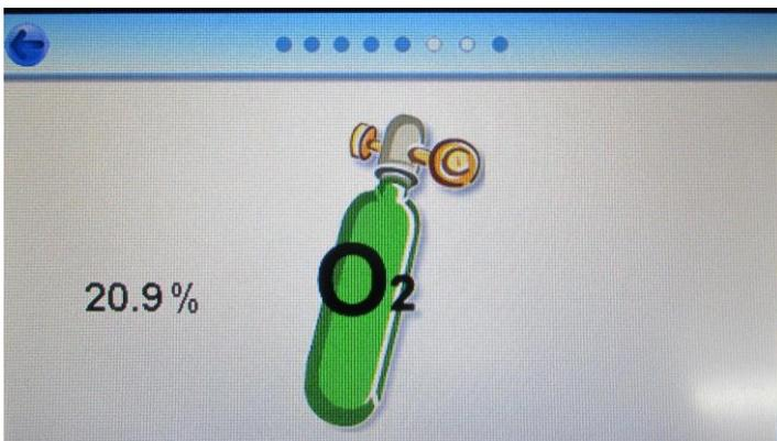
The instrument will then change operating modes to continuously display the Oxygen reading, connect your air source and the instrument will continue to provide a reading until you press the arrow key in the top corner.
