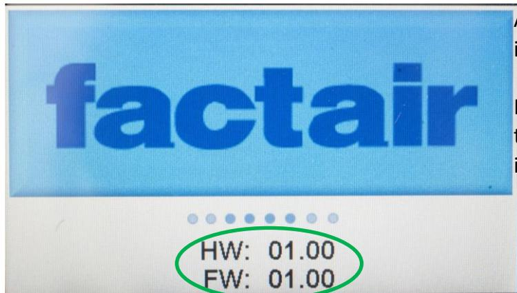
A splash screen will be displayed which shows the instruments hardware and firmware versions.
