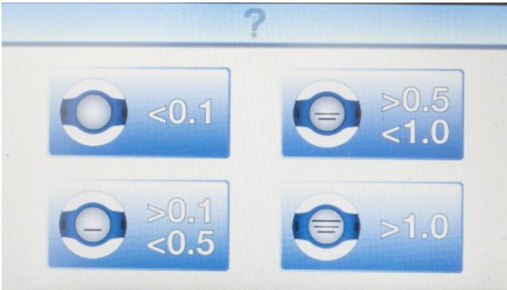
Once the test is complete close the flow control valve, the readings from the Impactor can now be entered.
