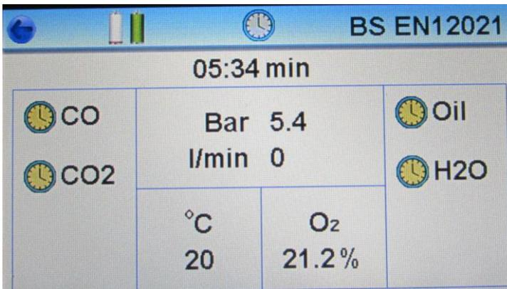
The test will now commence and the duration will be displayed as a countdown, together with pressure, flowrate, ambient temperature and oxygen content.
