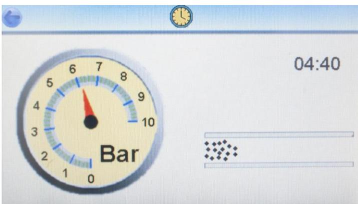
The instrument will now commence a 5-minute purge sequence, during which time an airflow will be passed through the test ports and across the electronic cells. This clears contaminants from previous tests and ensures that a representative sample is being tested.
