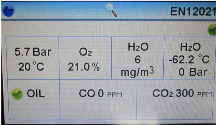
The “test complete” screen displays all the measurements recorded during the test. And automatically determines whether the test was a pass or fail against the standard displayed in the top right corner of the screen. For water content on high pressure tests both the measured value in mg/m<sup>3</sup> and the atmospheric dewpoint are provided.
