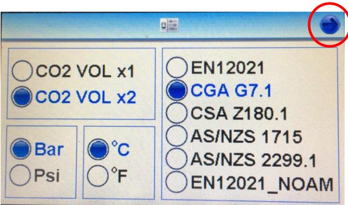
In this menu you can then choose the following; CO<sub>2</sub> sample rate, pressure and temperature units of measure and the breathing-air test standard.
