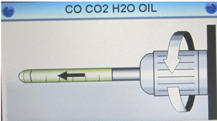
Once the purge has finished, the Water (F4500 only), CO, CO<sub>2</sub> and Draeger Impactor/oil tubes should be inserted into the test ports and tightened firmly; ensure the Impactor has an intact protective seal.
