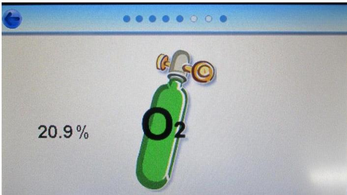
The instrument will then change operating modes to continuously display the oxygen reading, connect your air source and the instrument will continue to provide a reading until you press the arrow key in the top corner.
