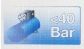
Select (Airline < 40 bar) – note the maximum pressure the instrument is rated to is 10 bar.
