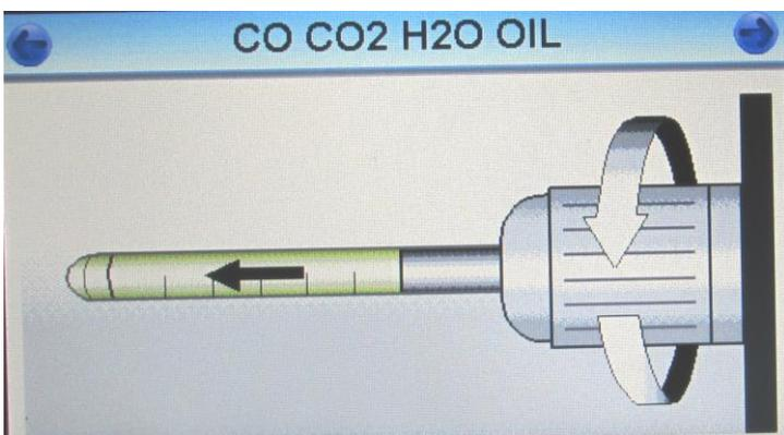
Once the purge has finished, the Water (F4500 only), CO, CO<sub>2</sub> and Draeger Impactor/oil tube should be inserted into the test port and tightened firmly; ensure the Impactor has an intact protective seal.
