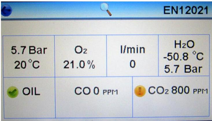
If the test was a fail an orange exclamation mark would be indicating those criteria which did not meet the standard. The photograph opposite is an example of a failed test where carbon dioxide failed to meet the requirements of the selected standard.
