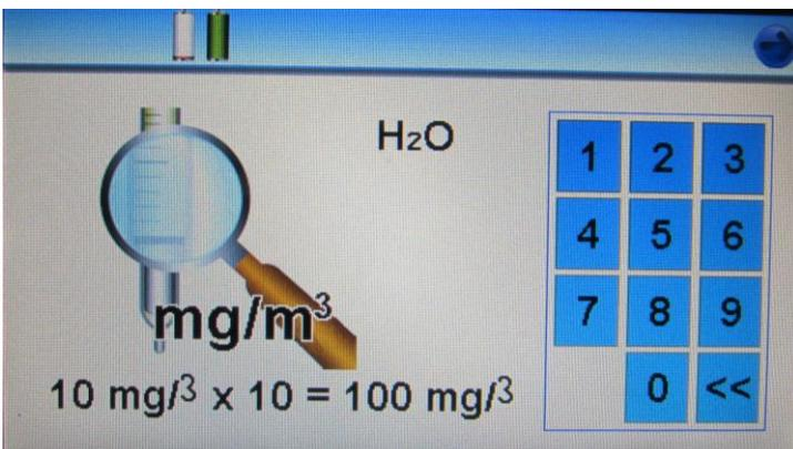
For the water tube reading there is an on-screen note if you selected the 50 to 2000mg/m<sup>3</sup> scale to confirm that the reading you enter will be automatically multiplied by 10 to provide the corrected result for this range.
