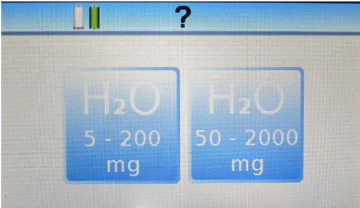
The F4500 can be configured with the Draeger 6728531 water tube for 2 different scales. Select the appropriate water range: 5 to 2000 mg/m<sup>3</sup> is for standard airline systems with a fridge dryer or no dryer and 5 to 200 mg/m<sup>3</sup> is for systems incorporating desiccant dryers. Having selected the appropriate range press the arrow key. (This screen will not appear on the F4500ED)
