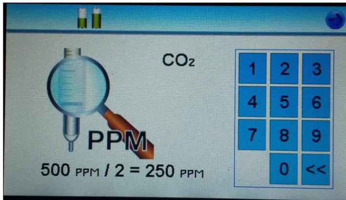
When entering the test results into the tester, the tube reading shall automatically be divided by two, to reflect the actual reading as shown here.
