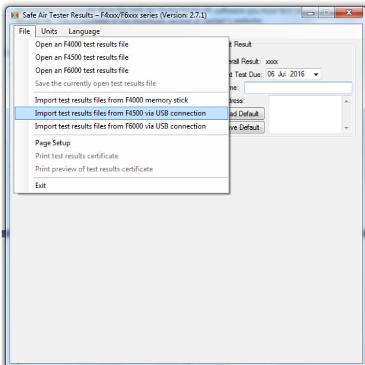
Then click on the File drop down menu and select import test results from F4500 via USB connection.
