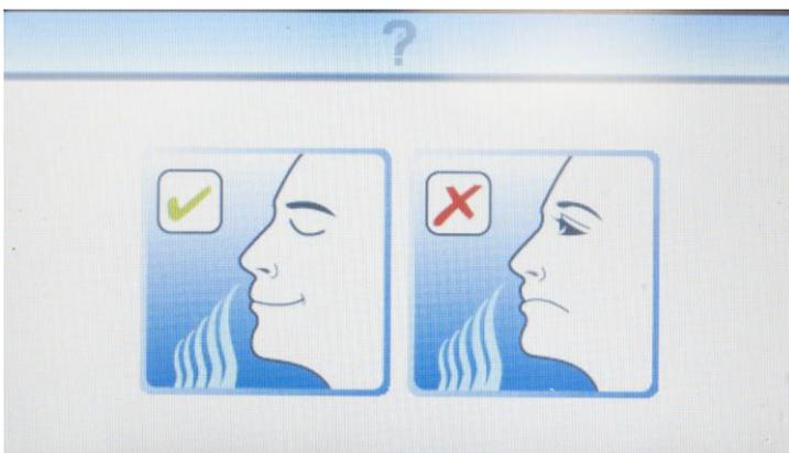
Carry out the odour test by gently opening the flow control valve and smelling the air exhausted from the sintered outlet, then close the valve. If there is a serious odour problem, fail the sample at this point of the test. Initiating flows of seriously contaminated air through the tube ports could result in damage to the unit. If the odour test is satisfactory, press the 'pass' icon.
