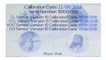
A stylus pen is provided for use with the touch screen. The display will show the calibration date, serial number and check the status of each sensor. Once each sensor status has been checked follow the touch screen prompt on screen to proceed.
