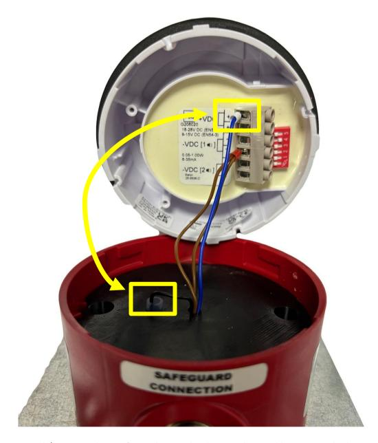
The alarm sound / tone can be configured using the dip switches and by moving the brown wires between VDC 1 and VDC 2.
