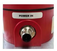
3. Fit the connection cable between the FAC0966 and SafeGuard.
