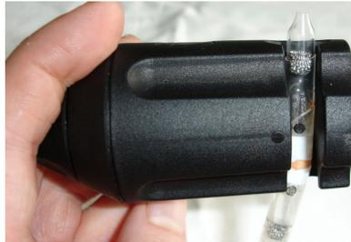
3. Place your used detector tubes in the F2154 Travel Container, until they can be disposed of properly as "sharps" or glass.
