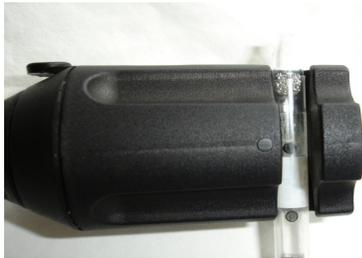
2. With one hand holding the cutter, the other holding the tube and with your thumb against the base of the cutter, apply pressure to the tube, this should break the inner tube.
