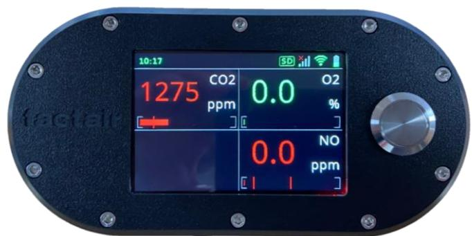
The SafeGuard can be configured using a local WiFi connection which is available from a smart phone/tablet device; this allows alarm readings and datalogging interval to be set. The datalog can also be downloaded as a CSV file and includes the minimum, maximum and average sensor reading during the user selected datalogging interval.
