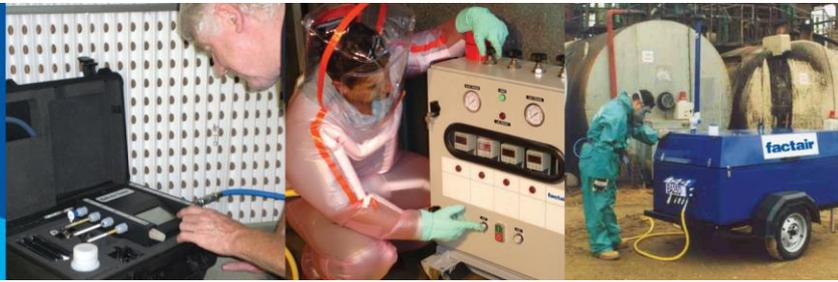
The SafeGuard is the latest addition to the Factair test instrument range. This configurable instrument is available for monitoring either atmospheric or compressed-air supplies (up to 10 barg). Up to 6 different sensors can be fitted to suit a client's individual requirements. As standard the compressed-air version is fitted with a dewpoint meter rated down to  $-20^{\circ}\text{C}$  PDP.
