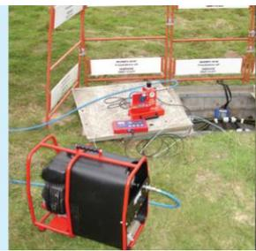
The Factair FM17 is the ideal compressor for mini cable blowing in small ducts up to approximately 14mm. The Kaeser M17 is specially modified by Factair with the addition of an aftercooler and water separator, reducing the compressed-air temperature to within 10°C of the ambient temperature. All condensate removed is re-vapourised back to atmosphere via the engine exhaust system. This self contained unit then avoids the need for separate ancillary aftercoolers and extra connection hoses.
